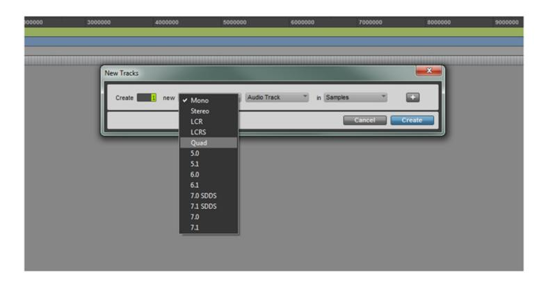
A single Quad track is all that is required in order to playback SoundField B-Format and A-Format and insert the plug-in. This will however require your SoundField B-Format or A-Format to be in a single four channel wav file, if this is not the case you can either bounce four mono tracks into a single four channel file or you can route four mono tracks to a Quad Aux track in which you can then insert the plug-in.
