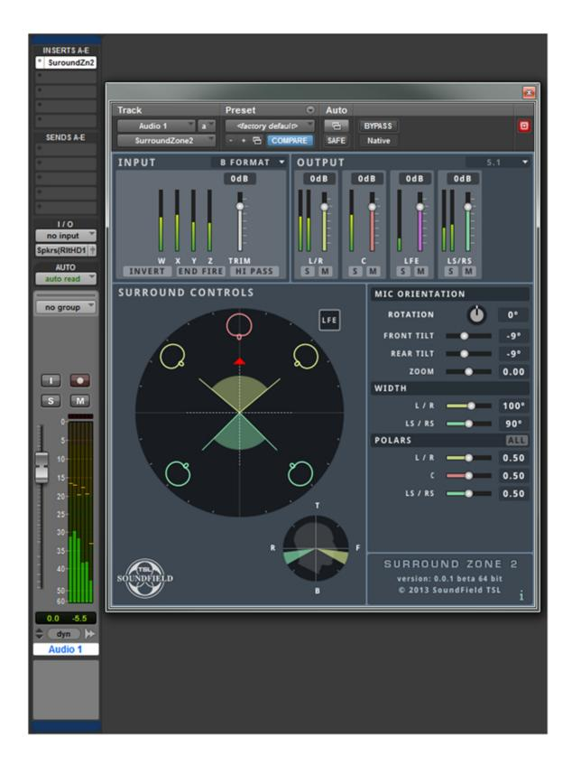
The screenshot above shows how a 5.1 output version of the plug-in has forced the output of the "Quad" track to a 5.1 output. We are now all set and ready to start playing with the controls.
