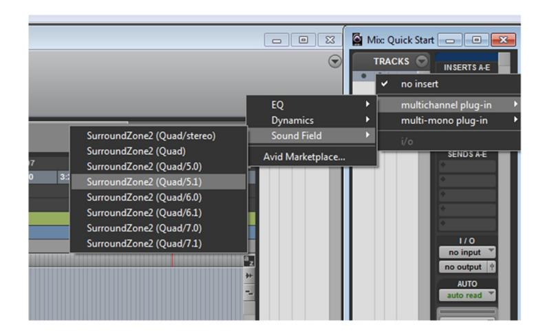
SurroundZone2 is available in a variety of output formats and these are simply selected from the plug-in insert drop down menu. The available output formats are: Stereo, B-Format (for A-Format input only), 5.0, 5.1, 6.0, 6.1, 7.0 and 7.1.
