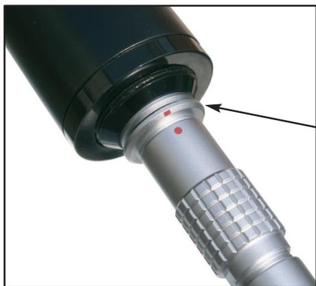
Push silver disc on microphone base at the 'red dot' position to release connector.
