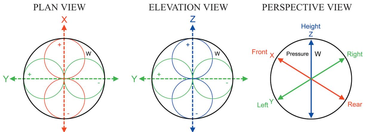
X: HORIZONTAL VECTOR: FRONT/REAR PRESSURE-GRADIENT COMPONENT
