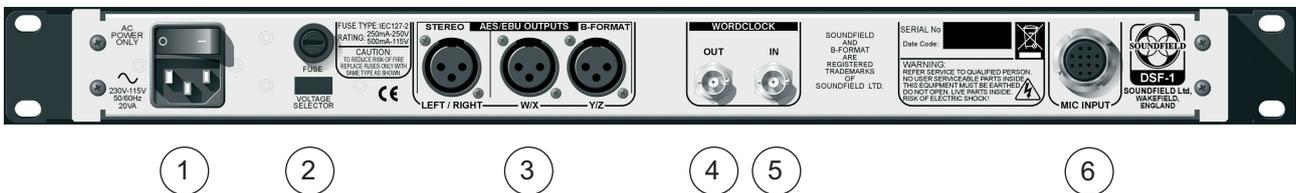
**1. MAINS POWER** - ON/OFF mains power switch / IEC mains power inlet.
