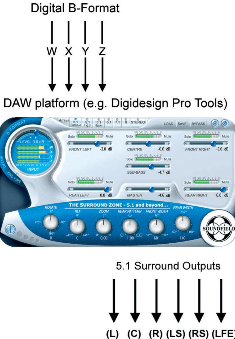
The SoundField Surround Zone software plug-in is designed to accept the four B-Format signals (W, X, Y & Z) generated by the DSF-1. All plug-in features can be utilised either retrospectively in the studio after the recording has taken place or ‘live’ and provides the user with the most powerful stereo and surround sound recording/post-production package available.
