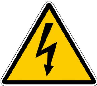
The lightning flash with arrow head symbol within an equilateral triangle is intended to alert the user to the presence of dangerous voltages and energy levels within the product's enclosure that may be of sufficient magnitude to constitute a risk of electric shock or injury.
